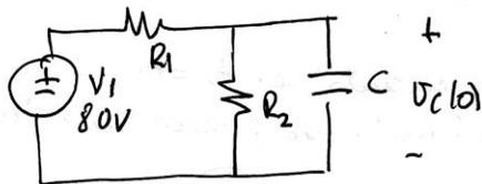
$$V_c(0) = \frac{V_1 R_2}{R_1 + R_2} = 50V$$
