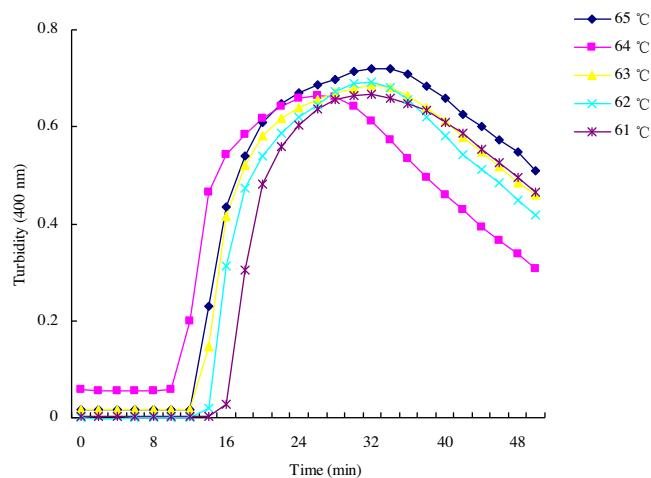
**Fig. 3.** Effect of different RT-LAMP reaction temperatures in ZIKV detection.
